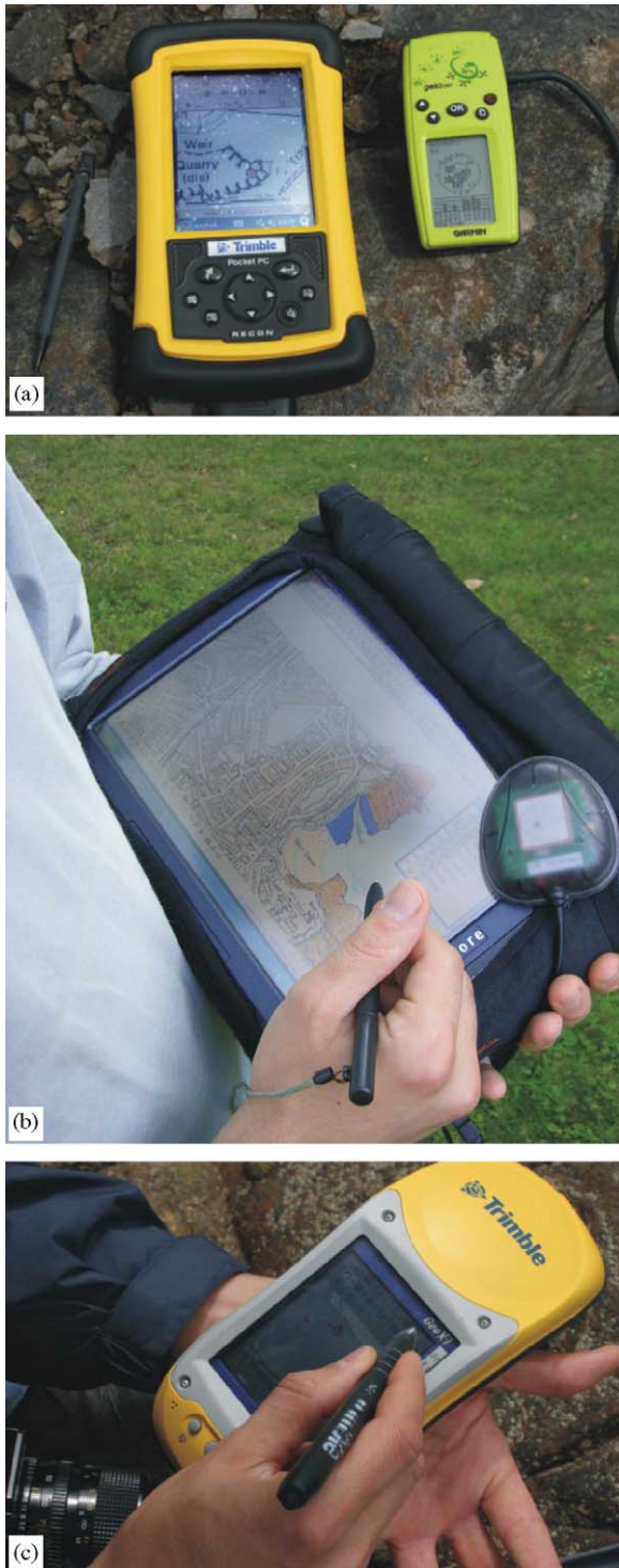
Fig. 1. PDA and tablet PC systems compared: (a) Trimble Recon PDA running ArcPad software with Garmin Geko 201 GPS; (b) Xplore tablet PC running Map IT software with Hicom HI-204S GPS receiver and (c) Trimble GeoXT integrated PDA and GPS receiver running ArcPad software.
